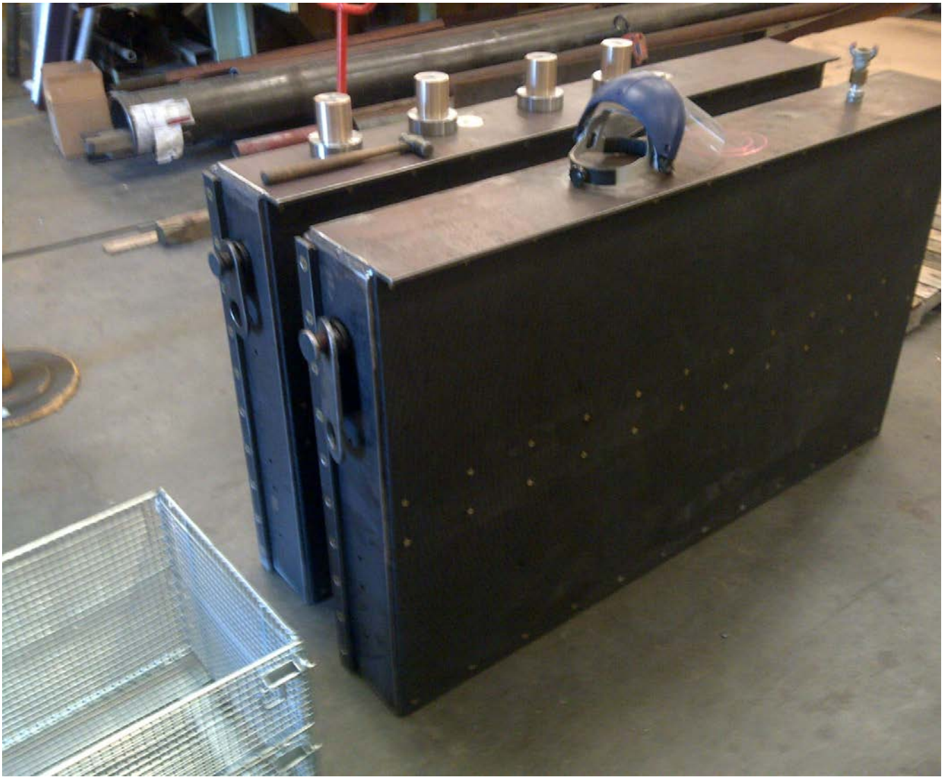
Progress on new 159 weir construction. Remaining work; Seal install, wheel install and paint.
